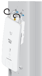
Connecting to a Sector Antenna
