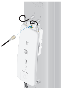
Connecting the GPS Antenna
