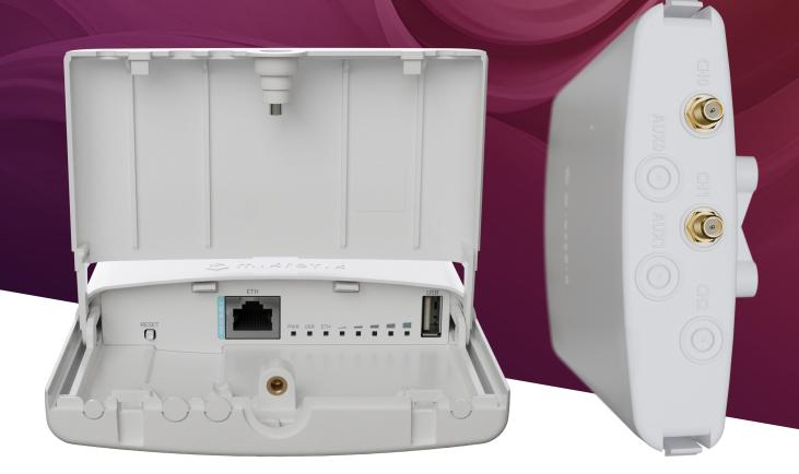
This weatherproof board features a modern Qualcomm Maple CPU based on the ARM architecture, 256 MB of RAM, a USB port for extra storage or other needs, and a Gigabit Ethernet port with PoE-in.
