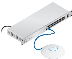
UniFi Switch with PoE Power Connection Diagram
